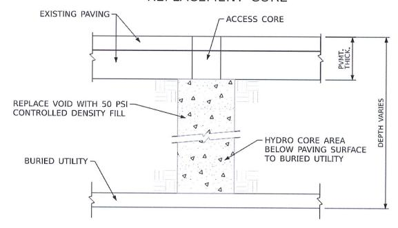
SPECIFICATION FOR THE CONSTRUCTION OF PAVEMENT CORE RESTORATION ENGINEERING DEPARTMENT CITY OF DES MOINES
