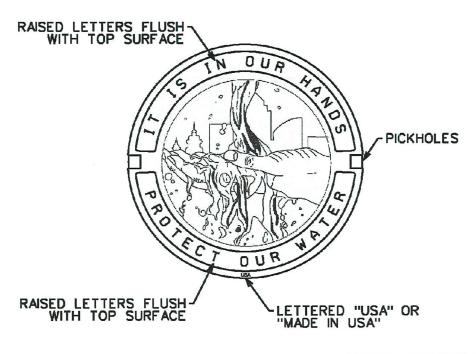
MATERIAL: CAST GRAY IRON ASTM A-48, CLASS 35B FINISH: NO PAINT
