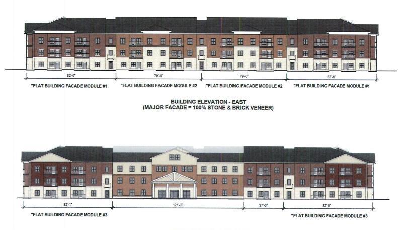
BUILDING ELEVATION - WEST (MINOR FACADE = 60% STONE & BRICK VENEER - 40% VINYL SIDING )
