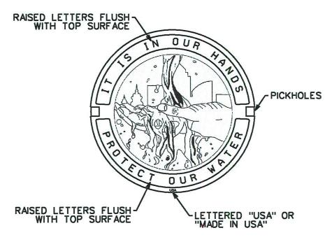
MATERIAL: CAST GRAY IRON ASTM A-48, CLASS 358 FINISH: NO PAINT
