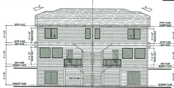
UNIT A-L UNIT A-R REAR ELEVATION SCALE: 1/8"=1'-0"
