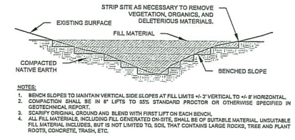
4 TYPICAL FILL SECTION Not to Scale
