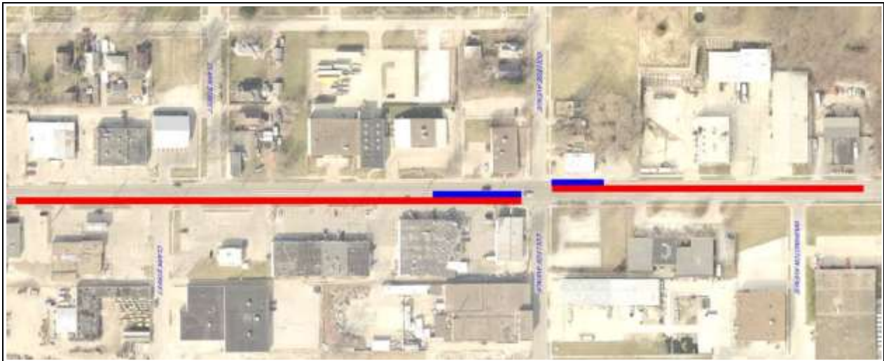
Queue Lengths at 2 nd Avenue and College Avenue Blue = 4-lane road, current traffic; Red = 3-lane road, current traffic
